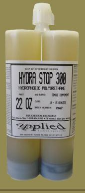
Hydra Stop 300 is a single component urethane foam grout used to stop water penetration. Upon contact with water Hydra Stop 300 foams and expands in volume to fill cracks, voids and honeycombs in concrete.
