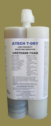
A-Tech T-Dry is a low viscosity hydrophilic urethane foam grout used to stop water leaks in concrete cracks. Its recommended use is in areas that will not dry out or in cracks with high rates of water penetration. This foam completely fills the defective area. After reacting, the finished foam is a highly flexible closed cell foam that prevents water penetration.
